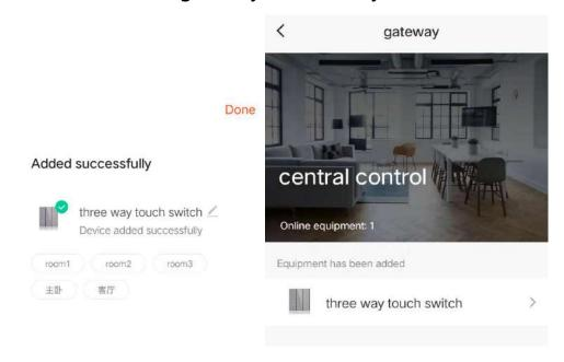
(8) You could change the device type by getting into the device interface in the App. It means the switch is off when it is in grey, and the switch is on when it is in green. You could also set up timers(Schedule) for the switches to realize the automation control.
