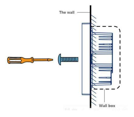
Depth of the wall box should be more than 50mm.
